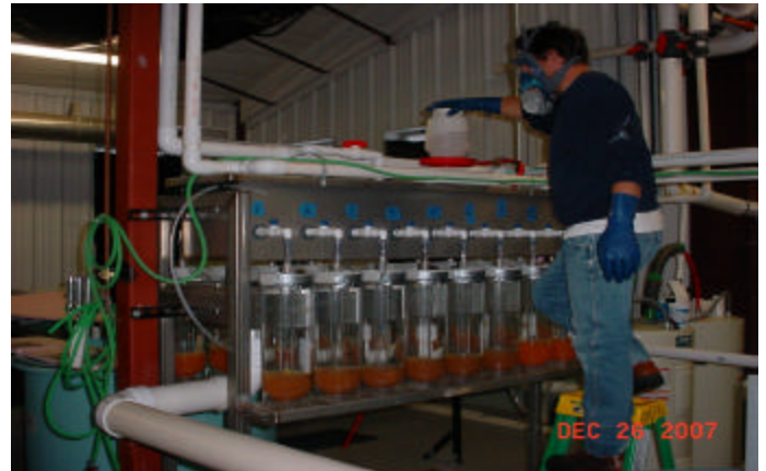
Kendall Holmes, Advanced NADF Technician placing a common chicken waterer modified for a 15 minute formalin drip treatment on lake herring eggs in a Bell Jar Incubation system.
